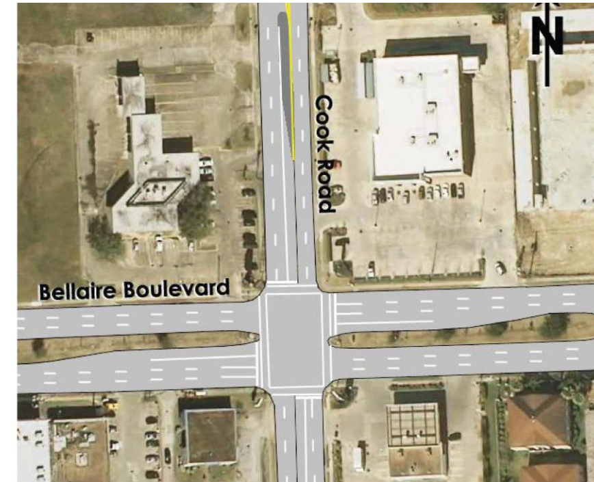
Bellaire Boulevard at Cook Road Proposed Intersection Layout
